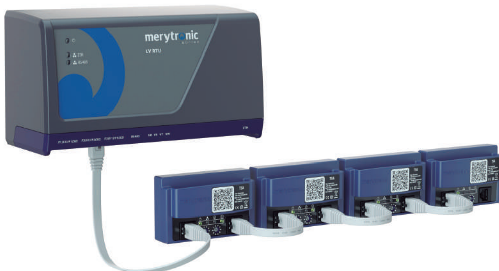
Daisy chain connections
